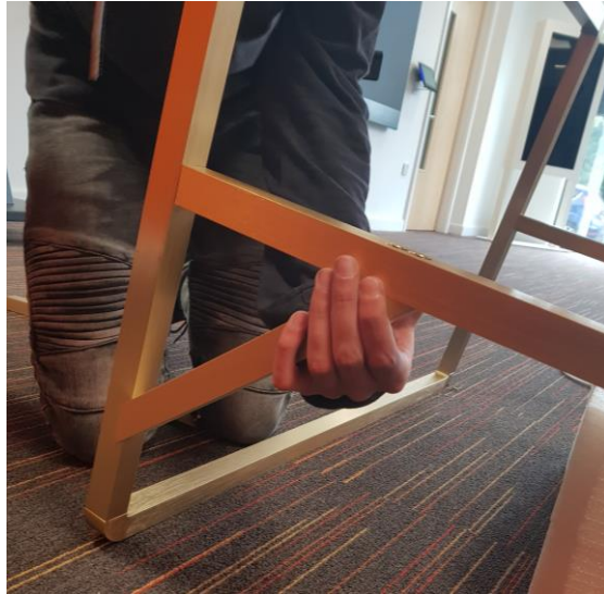
Figure 7 Screwing "E" Parts onto "A" Parts and base
